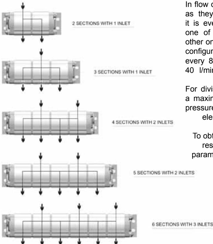
In flow dividers with many inlets, as they are all communicating it is even possible to use only one of them, by plugging the other ones. We suggest to make configurations with one inlet every 80 l/min (for 2DRE) and 40 l/min (for 1.5DRE) of flow elaborated.
