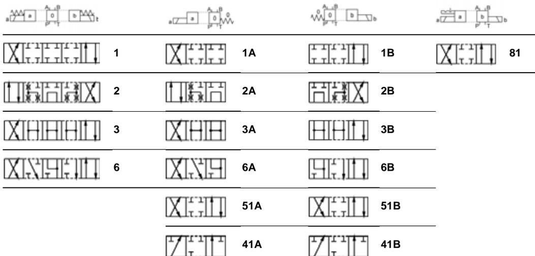
Port T in the valves with spool type 41A and 41B to be used as leakage line.
