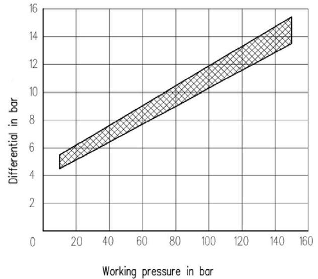
DIFFERENTIAL PRESSURE OF IP-350 PRESSURE SWITCH
