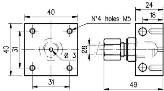
It allows the pressure switch mounting:
