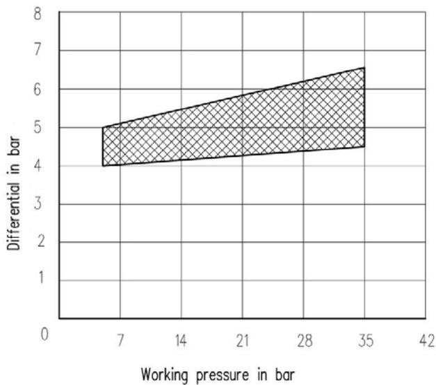
DIFFERENTIAL PRESSURE OF IP-150 PRESSURE SWITCH
